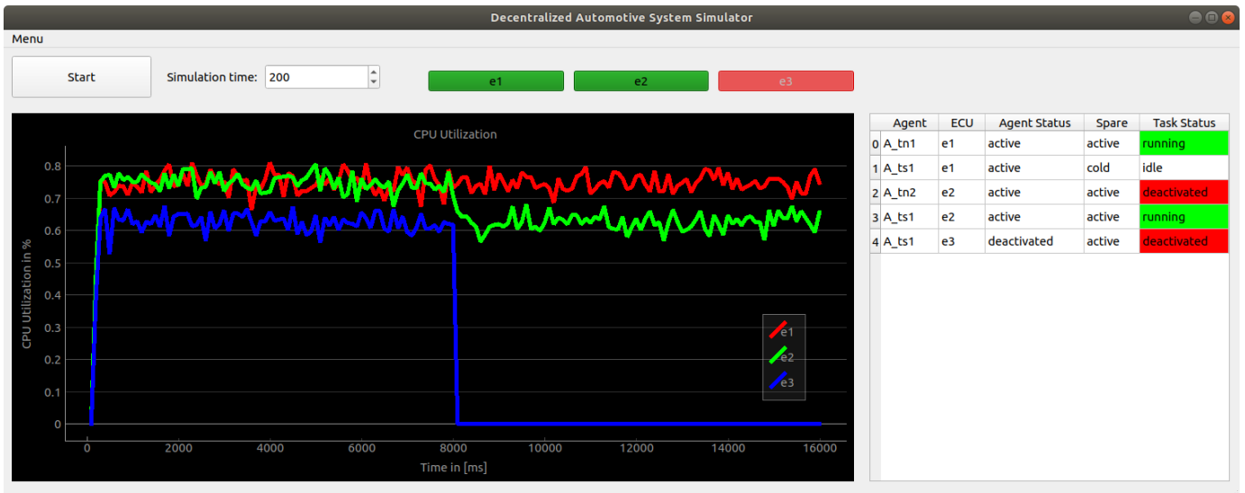
Figure 2: Simulation framework performing simulation of the example described in Figure 1. The plots show the CPU utilization of the three ECUs e_1 (red), e_2 (green), and e_3 (blue). The table on the right displays the situation at the end of the simulation. After the failure of ECU e_3 at 8000ms , task t_{s1} restarted on ECU e_2 , leading to the shutdown of t_{n2} . As t_{s1} requires slightly less resources than t_{n2} , the change can be examined in the plot.
