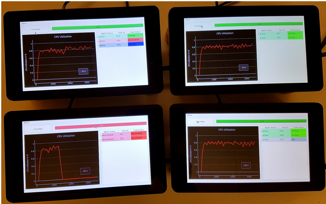
■ Figure 2 Our demonstrator setup consisting of 4 Raspberry Pis, which are connected over a switch and Ethernet links. Each of the hardware nodes is running a single simulation instance with our agent-based graceful-degradation approach from [5]. The graphical user interface presents the simulated CPU utilization and the status of the agents and tasks.
